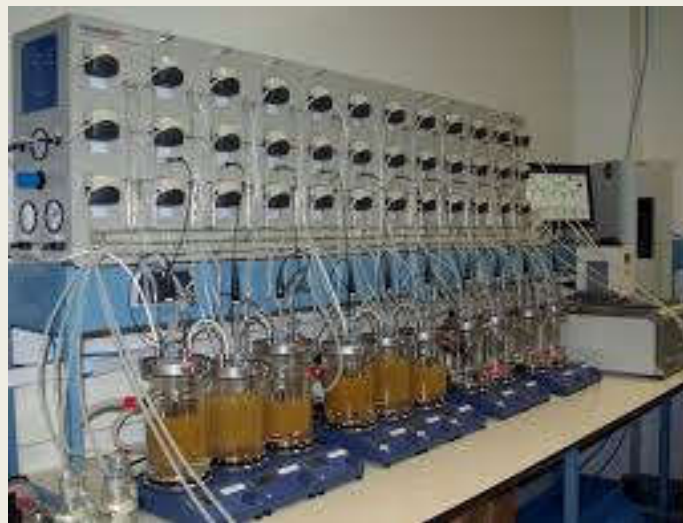
Simulator of Human Intestinal Microbial Ecosystem (SHIME®)
